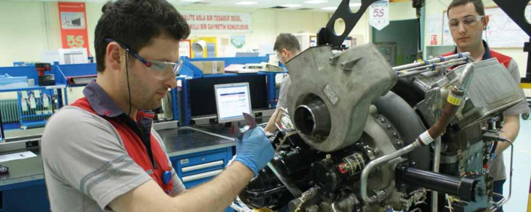
The studies were conducted in order for "Cooling Fan" component used in APS3200 APUs to be repaired and tested within Turkish Technic Inc. and the testing bench was designed and manufactured by the Directorate of Design and Development. For "Curvic Coupling Runout" controls of a group of rotating parts of APUs, which are within the capability of shop, the testing bench was designed and tendered out by the Directorate of Design and Development.
