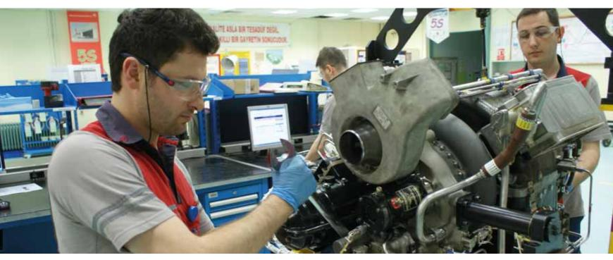
The studies were conducted in order for "Cooling Fan" component used in APS3200 APUs to be repaired and tested within Turkish Technic Inc. and the testing bench was designed and manufactured by the Directorate of Design and Development. For "Curvic Coupling Runout" controls of a group of rotating parts of APUs, which are within the capability of shop, the testing bench was designed and tendered out by the Directorate of Design and Development.
